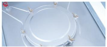
Robust transport frame for protection of interior tank Crane openings in frame supports for fixing of lifting beams of crane hooks. Deep drawn top head and bottom assure high form stability Screw cover with hinge closing by 6 hammer bolts with wing nuts Pressure relief valve UH/D2 (latest opening at +0.65 bar)
