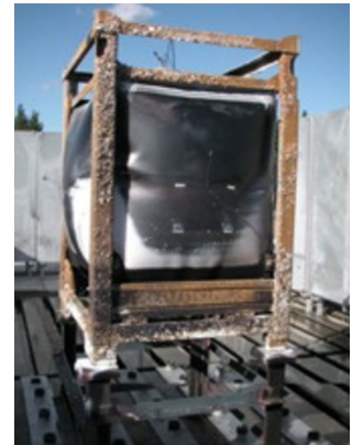
Stainless steel IBC after a fire test
